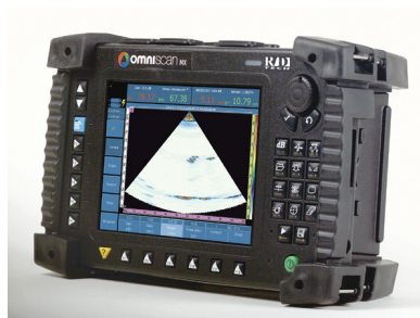
Figure 1 - Photo of Olympus NDT OmniScan performing an L-wave S-scan.
